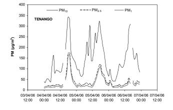
**Fig. 6.** Hourly PM levels measured at the rural site Tenango, showing the Mexico City's plume impact causing high levels of PM<sub>1</sub>.
