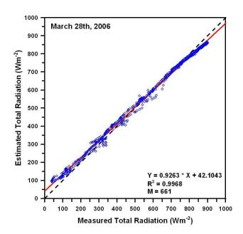
**Fig. 6a.** Estimated vs. measured values of total solar radiation on horizontal surface for Athens on 28 March 2006. The best fit equation (red line), the determination coefficient value ( $R^2$ ) and the number of available data (M) are also given. The y=x (dashed) line shows the ideal case of complete agreement between estimated and measured values.
