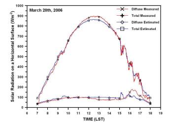
Fig. 4a. Comparison between MRM simulations (blue lines) and measurements (red lines) for Athens on 28 March 2006.
