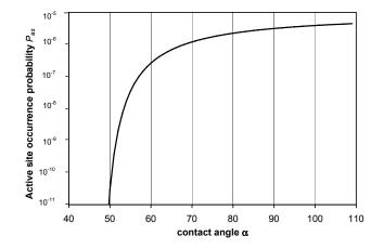
Fig. 6. Occurrence probability of active sites as a function of contact angle  $\alpha$ . This function was used to calculate the freezing curves in Figs. 4d and 5d.
