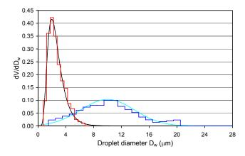
**Fig. 1.** Normalized volume distribution of water-in-oil emulsions: microscopically determined distributions are given in red (small droplets) and dark blue (large droplets), fitted functions in black (lognormal distribution, small droplets) and light blue (normal distribution, large droplets).
