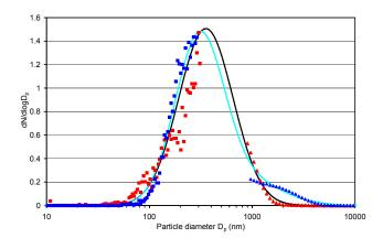
**Fig. 2.** Normalized number distributions of Arizona Test Dust (ATD): measured size distributions are given in red (fine ATD; squares: scanning mobility particle sizer (SMPS), triangles: aero-dynamic particle spectrometer (APS)) and dark blue (coarse ATD; squares: SMPS, triangles: APS). Fitted distributions are in black (fine ATD) and light blue (coarse ATD).
