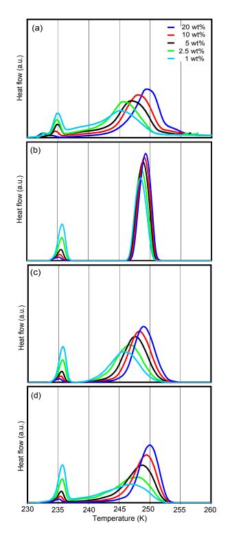
Fig. 5. Ice nucleation of coarse ATD. (a) DSC freezing experiment of emulsified aqueous suspensions of coarse ATD with concentrations from 1-20 wt%. (b) Modeled freezing curve with a constant contact angle of 65°. (c) Modeled freezing curve with a lognormal size distribution of contact angles. (d) Modeled freezing curve with nucleation occurring on active sites.
