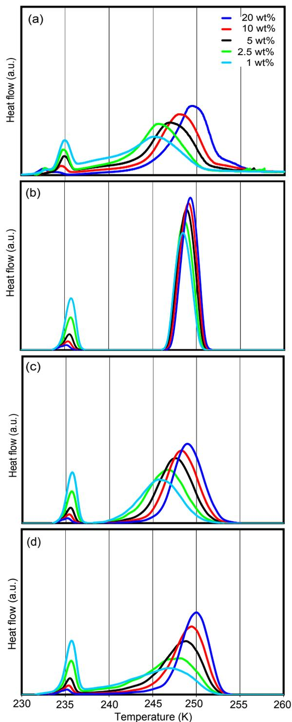
**Fig. 5.** Ice nucleation of coarse ATD. **(a)** DSC freezing experiment of emulsified aqueous suspensions of coarse ATD with concentrations from 1–20 wt%. **(b)** Modeled freezing curve with a constant contact angle of  $65^\circ$ . **(c)** Modeled freezing curve with a lognormal size distribution of contact angles. **(d)** Modeled freezing curve with nucleation occurring on active sites.
