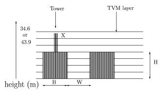
**Fig. 3.** Configuration of the 1-D model, with forcing from the top (X), and calculation down to the ground in the street canyon (x), and schematic representation of the city (street and buildings) in the urban module with height of the buildings H, width of the buildings B, and width of the street W.
