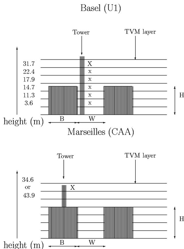
**Fig. 3.** Configuration of the 1-D model, with forcing from the top (X), and calculation down to the ground in the street canyon (x), and schematic representation of the city (street and buildings) in the urban module with height of the buildings  $H$ , width of the buildings  $B$ , and width of the street  $W$ .
