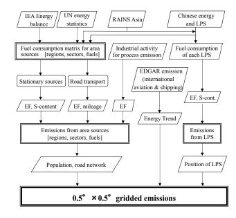
**Fig. 2.** Flow chart for the estimation of emissions.
