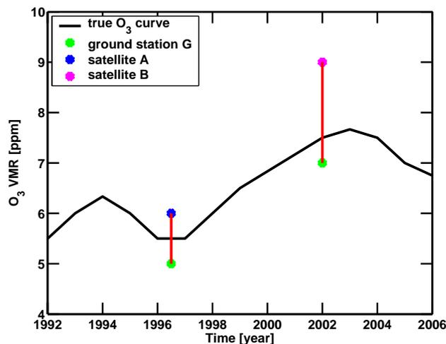
Fig. 13. Scheme of cross-validation by double differencing: Measurements of satellites  $A$  and  $B$ , separated in time, are compared by using the long-term data set of ground station  $G$  (the satellite measurements are nearby the ground station). The difference of lengths of the red lines is estimated to be the difference of the systematic errors of the satellites  $A$  and  $B$ . The black curve is the unknown time series of true ozone at a fixed altitude over the ground station.
