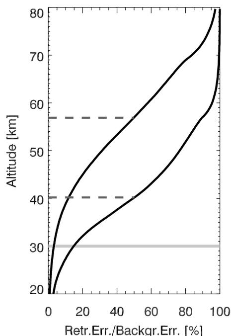
**Fig. 1.** Retrieval-to-background temperature error ratio profiles (in percent,  $100 \cdot q_r$ ) for two cases corresponding to approximately the upper and lower limits of  $q_r$  in CCR (more details and exception see text).  $hq_{50}$  is indicated by dark-grey dashed lines, the 30 km level by a light-grey solid line.
