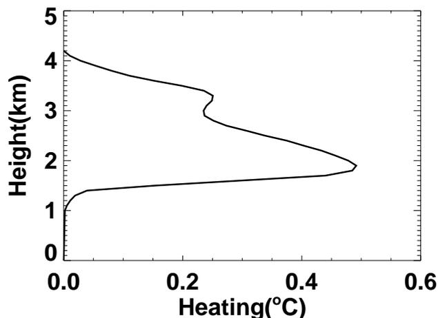
**Fig. 2.** The heating profile by dust layers used in the simulations (Based on Cheng et al., 2002).
