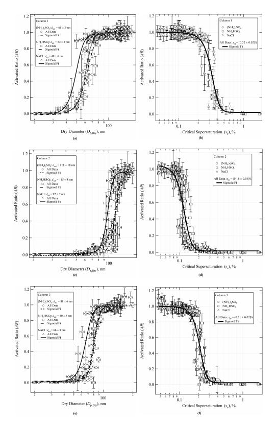
Fig. 6. Calibration curves for column 1 (panels  $\mathbf{a}$  and  $\mathbf{b}$ ), column 2 (panels  $\mathbf{c}$  and  $\mathbf{d}$ ), and column 3 (panels  $\mathbf{e}$  and  $\mathbf{f}$ ) using  $(NH_4)_2SO_4$ ,  $NH_4HSO_4$ , and NaCl as calibration salts.
