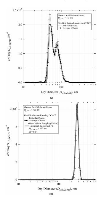
**Fig. 11.** DACAD size distributions for DMA size-selected particles with (a)  $D_{p,DMA}$ =145 nm and (b)  $D_{p,DMA}$ =300 nm.
