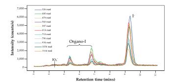
**Fig. 3.** IC-ICP-MS chromatogram of iodine species in snow. Iodate less than 0.3 nmol/l. Largest iodide peak 11.4 nmol/l.
