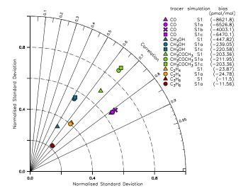
**Fig. 25.** Taylor diagram of the comparison between aircraft measurements and model results. The color code denotes the tracers and the symbols denote the different sensitivity simulations, respectively. The empty box represents the measurements. The biases are listed in parentheses (in pmol/mol).
