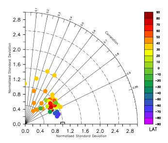
**Fig. 6.** Taylor diagram comparing 7 year (1998-2004) monthly averages of CO from the model simulations with the surface observations from the NOAA/CMDL network (Novelli et al., 1998). The colour code denotes the geographic latitude.
