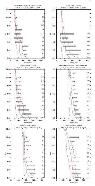
**Fig. 8.** Vertical profiles of CO (nmol/mol) for some selected campaigns from Emmons et al. (2000). Asterisks and boxes represent the average and the standard deviation (w.r.t. space and time) of the measurements in the region, respectively. The simulated average is indicated by the red line and the corresponding simulated standard deviation w.r.t. time and space by the dashed lines. On the right side the number of measurements is listed.
