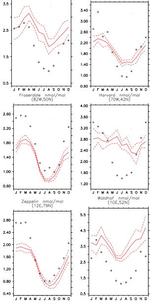
**Fig. 10.** Seasonal cycle (monthly averages) of C<sub>2</sub>H<sub>6</sub> (in nmol/mol) for some selected locations at the surface (Solberg et al., 1996). Model: red solid line; model standard deviation: red, dashed line; measurements: circles.
