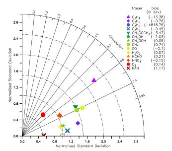
**Fig. 2.** Taylor diagram of the comparison between aircraft measurements and model results, both weighted with relative uncertainties (Jöckel et al., 2006). The biases are listed in parentheses (units of standard deviation). The empty box represents the measurements.
