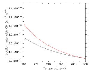
**Fig. 16.** Temperature dependence of the reaction coefficient  $(cm^3s^{-1})$  for  $C_3H_6+OH$  according to the IUPAC recommendations (black: Atkinson et al., 2005; red: Atkinson et al., 1999).
