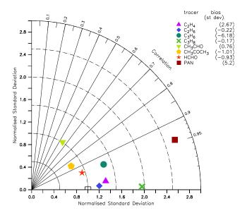
**Fig. 4.** Taylor diagram of the comparison between station measurements and model results, both weighted with relative uncertainties. The biases are listed in parentheses (units of standard deviation). The empty box represents the measurements.
