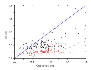
**Fig. 32.** Scatter plot of model results versus observations of  $CH_3OH$  (both in nmol/mol). The red circles represent the results of the reference simulation (SI), the black triangles those of the sensitivity simulation (SIa).
