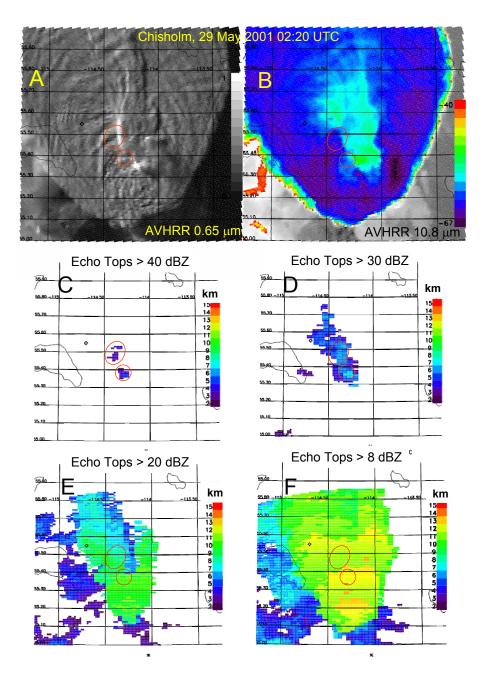
**Fig. 13.** The relations between radar and cloud features of the phase-2 Pyro-Cb at 02:20 UTC. The AVHRR visible (**A**) and thermal IR (**B**) images are mapped on the same geographical grid as the radar echo top maps at thresholds of 40, 30, 20 and 8 dBZ (**C**-**F**). The red circles mark the areas of the most intense radar echoes >40 dBZ, shown in (C). Note that this area of strongest reflectivities is downwind of the upshear edge of the overshooting tower.
