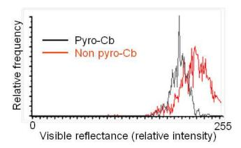
**Fig. 10.** Histogram of the visible reflectance levels at the flat part of the anvil top of a normal (red line) and pyro-Cb (black line). The histograms correspond to areas A and B from the pyro-Cb and normal Cb in Fig. 9, respectively. The reflectance values are in relative units ranging between 0 and 255. Note the significantly lower reflectance of the pyro-Cb.
