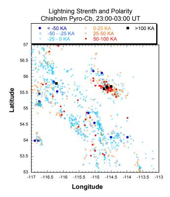
**Fig. 14.** The lightning strength [kiloAmpere] and polarity in the area that includes the pyro-Cb during the peak hours of the firestorm, 28 May 23:00–29 May 03:00 UTC. The lightning strokes with normal polarity (negative) are shown in blue, and the positive lightning strokes are shown in red, except for black squares that represent the strongest positive flashes. The Pyro-Cb can be clearly seen as the red aggregate of positive lightning.
