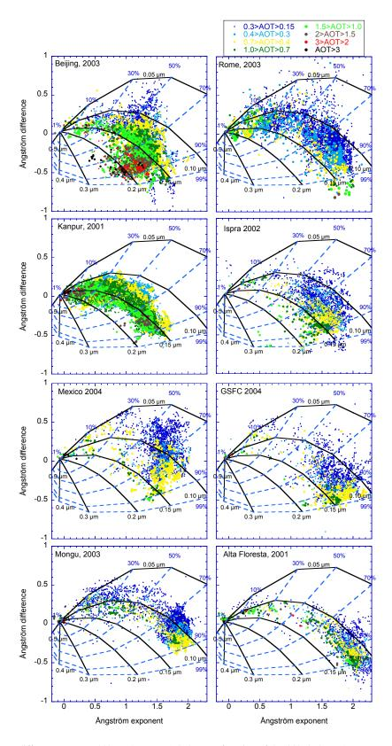
**Fig. 3.** Angstrom exponent difference,  $\delta\alpha = \alpha(440, 675) - \alpha(675, 870)$ , as a function of the 440–870 nm Angström exponent and AOT (color code) for eight AERONET stations (from top): Beijing (China), Rome (Italy), Kanpur (India), Ispra (Italy), Mexico City (Mexico), GSFC (USA), Mongu (Zambia) and Alta Floresta (Brasil). Only cloud-screened data with AOT>0.15 were used.
