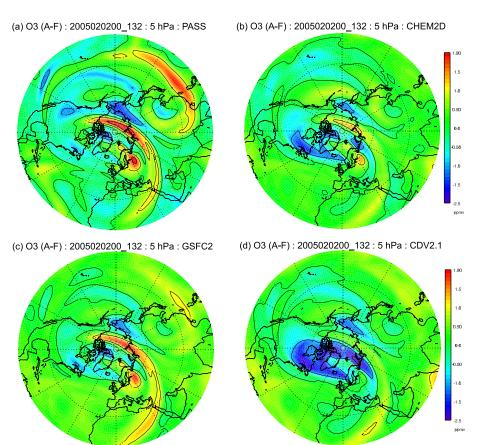
**Fig. 17.** Difference between ozone analysis (A) valid 12:00 UT on 7 February 2005 and forecast (F) mixing ratios (in ppmv) at 5 hPa from NOGAPS-ALPHA 132-h ozone hindcasts initialized 00:00 UT on 2 February 2005 using (**a**) no photochemistry (passive), the (**b**) CHEM2D-OPP, the (**c**) GSFC2, and the (**d**) CD86 V2.1 ozone photochemistry parameterizations. Polar projection extends to  $10^{\circ}$  N latitude.
