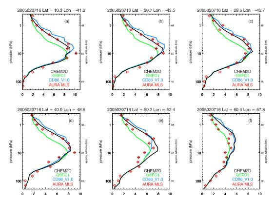
**Fig. 12.** A comparison of 135-h NOGAPS-ALPHA ozone hindcasts (in ppmv), initialized at 00:00 UT on 2 February 2005 and valid 15:00 UT 7 February using CHEM2D-OPP photochemistry (black curve), CD86 V1.0 photochemistry (blue curve), original GSFC1 photochemistry (green curve), and Aura MLS ozone profile measurements (red diamonds) along the 16:00 UT MLS flight track indicated in Fig. 10.
