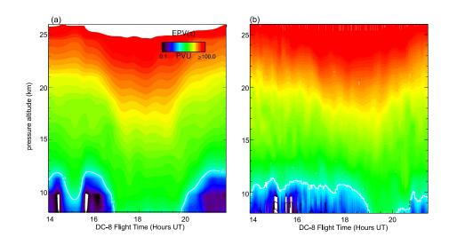
**Fig. 21.** Cross section of Ertel's potential vorticity in potential vorticity units (PVU) along the DC8 flight path of 7 February 2005, derived from (a) NASA GMAO meteorological analyses (data courtesy of NASA Goddard Space Flight Center, Code 613.3), and from (b) 138-h T239L60 NOGAPS-ALPHA hindcast vorticity fields initialized 00:00 UT 2 February 2005 and valid at 18:00 UT 7 February. White contour denotes the 2 PVU contour indicating the approximate tropopause altitude.
