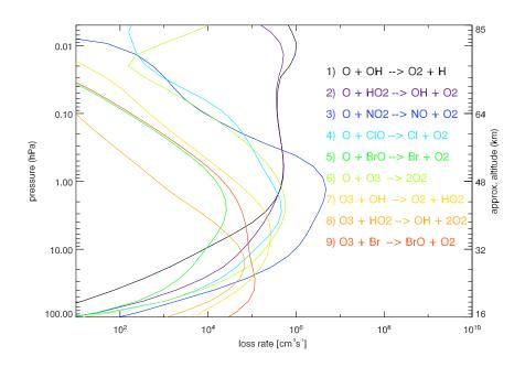
Fig. A1. Vertical profiles of individual CHEM2D odd oxygen loss rates (cm<sup>-3</sup>s<sup>-1</sup>) for 15 March over the equator, used to compute the photochemical relaxation time  $\tau_{O_3}$ .
