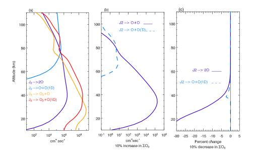
**Fig. A2.** (a) Vertical profiles of CHEM2D  $J_2$  and  $J_3$  photolysis terms for production of atomic oxygen in both ground state and excited state  $(O(^1D))$  for March conditions at 30° N; (b) the absolute reduction in  $J_2$  from (a) for an imposed 10% increase in overhead column ozone at each model vertical level; (c) as in (b) but for the percentage reduction in  $J_2$ .
