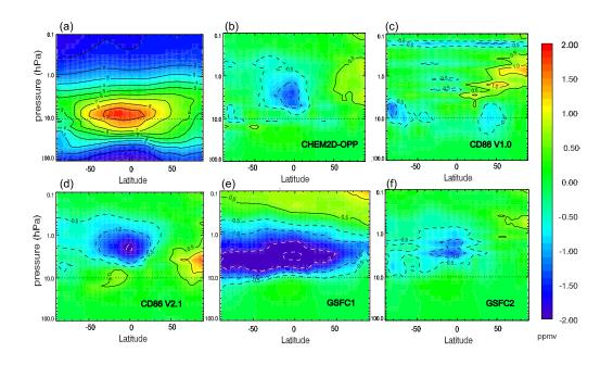
**Fig. 11.** (a) Zonal mean ozone mixing ratios (ppmv) at hour 144 of a NOGAPS-ALPHA hindcast using CHEM2D-OPP ozone photochemistry initialized at 00:00 UT 2 February 2005. Panels (b) through (f) plot the zonal mean difference between active and passive ozone mixing ratios computed from 144-h hindcast NOGAPS-ALPHA ozone fields using (b) CHEM2D-OPP, (c) CD86 V1.0, (d) CD86 V2.1, (e) GSFC1, and (f) GSFC2 ozone photochemistry parameterizations.
