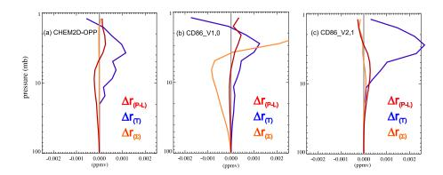
**Fig. 20.** Diagnostic calculations of  $\Delta r_{(P-L)}$  (red curve),  $\Delta r_T$  (blue curve), and  $\Delta r_{\Sigma}$  (orange curve) for the 135-h (15:00 UT) NOGAPS-ALPHA hindcasts at 50° N, 52° W, corresponding to Fig. 12e, using (a) CHEM2D-OPP, (b) CD86 V1.0, and (c) CD86 V2.1 photochemistry schemes.
