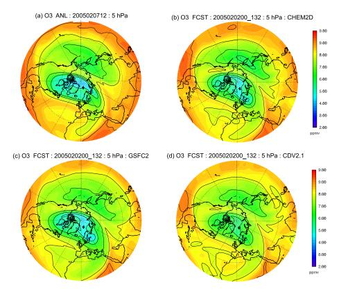
**Fig. 16.** Ozone mixing ratios (in ppmv) at 5 hPa from (**a**) the NASA GMAO ozone analysis valid 12:00 UT on 7 February, 2005, and NOGAPS-ALPHA 132-h ozone hindcasts initialized 00:00 UT on 2 February 2005 using (**b**) CHEM2D-OPP, (**c**) GSFC2, and (**d**) CD86 V2.1 ozone photochemistry parameterizations. Polar projection extends to 10° N latitude.
