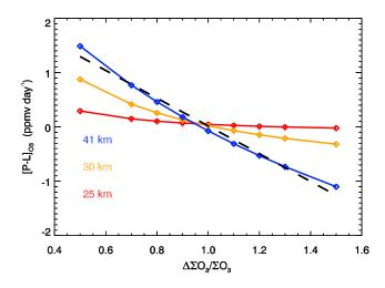
**Fig. 4.** The O<sub>3</sub> column ( $\Sigma$ ) dependence of CHEM2D (*P*-*L*) for perturbations of  $\pm$ 50% under March conditions at the equator.
