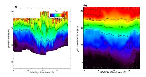
**Fig. 22.** Ozone mixing ratios in ppmv from (**a**) the AROTAL instrument aboard the NASA DC8 flight on 7 February 2005, plotted versus geometric altitude and from (**b**) a 138-h T239L60 NOGAPS-ALPHA ozone hindcast with CHEM2D-OPP photochemistry plotted versus geopotential height at locations along the DC8 flight track.
