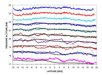
**Fig. 1.** Isentrope altitude cross-sections for an ER-2 flight from Hawaii to Fiji, 27 March 1994. The isentropes are 20 K of potential temperature apart starting with 400 K at  $\sim\!17.5\,\mathrm{km}$ . The ER-2 altitude is shown by the light-gray trace. The thick, smooth black traces are isentropes based on synoptic scale (assimilated) data. The thin colored traces, with detailed structure, are isentropes based on MTP/ER2 data.
