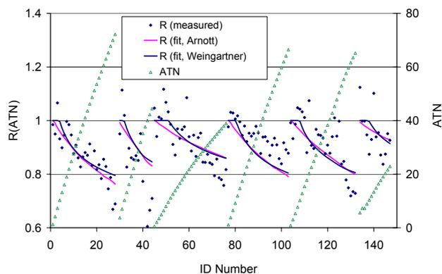
**Fig. 7.** Illustration of the effect filter loading (ATN, open triangles) on Aethalometer sensitivity ( $R$ ) for the 590 nm channel converted to 532 nm (data points were numbered consecutively). The measured sensitivity (solid diamonds) was fitted according to the expressions provided by Weingartner et al. (2003) (blue line) and Arnott et al. (2005) (magenta line).
