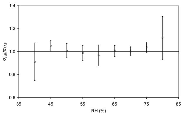
**Fig. 9.** The effect of relative humidity ( $RH$ ) on Aethalometer performance. Depicted are the mean and 95% confidence level of the ratios of ambient and dry absorption coefficients as measured by the Aethalometer ( $\sigma_{\text{aeth}}$ ) and the photoacoustic spectrometer ( $\sigma_{\text{PAS}}$ ), respectively.
