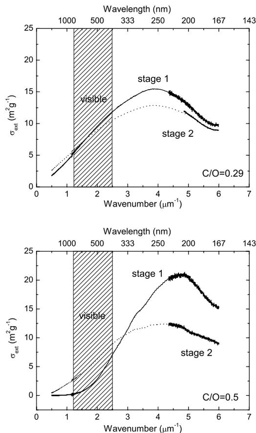
**Fig. 9.** Specific extinction cross sections corresponding to the samples produced with C/O ratios of 0.29 and 0.50 and deposited at the impactor stages 1 and 2. The smooth (noisy) traces represent measurements with the UV-VIS spectrometer (the VUV spectrometer). The combined spectra reveal the presence of a prominent band with a maximum in the  $3\text{--}5 \mu\text{m}^{-1}$  range. The visual range where the Ångström exponent was determined is shaded.
