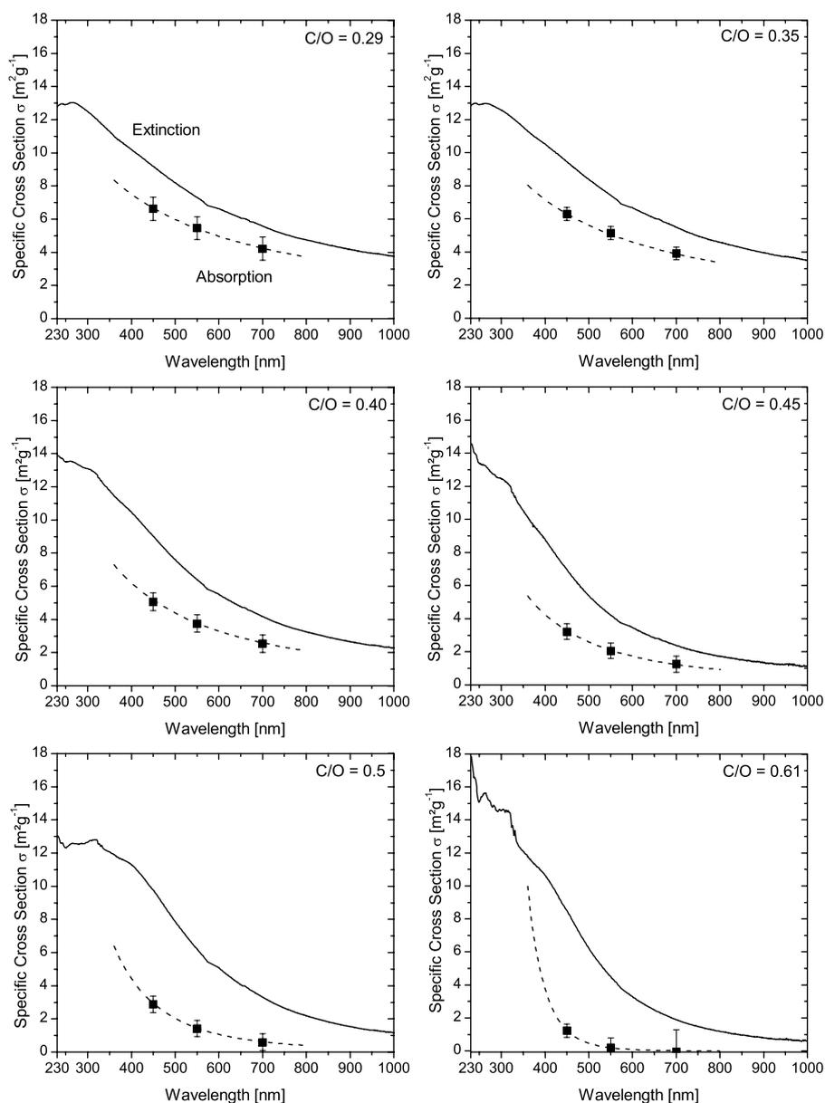
**Fig. 6.** Specific extinction (solid lines) and absorption (squares) cross sections derived for NAUA aerosol samples produced at different C/O ratios. The absorption values originate from extinction and total scattering (nephelometer) measurements (difference method, see Sect. 1). Dashed lines represent power laws fitted through the measured absorption cross sections.
