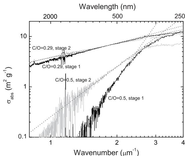
**Fig. 8.** Double logarithmic representation of the absorption behaviour in the visible range for samples produced at C/O ratios of 0.29 and 0.50 and deposited on impactor stages 1 and 2. The figure shows that the power-law behavior is no longer valid at wavenumbers larger than  $2.5 \mu\text{m}^{-1}$ .
