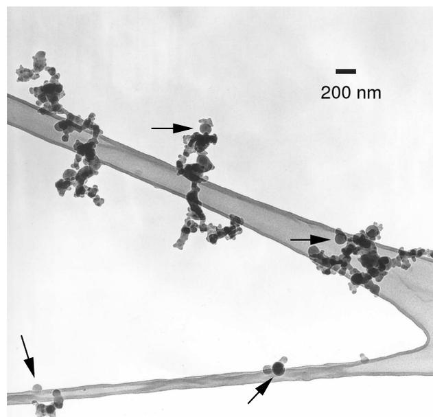
**Fig. 4.** TEM image showing the morphologies of carbonaceous aerosol particles produced at  $C/O=0.45$ . The arrows indicate larger spherical particles either isolated or attached to the soot aggregates. The long structures to which the particles are attached are bars of the supporting film.
