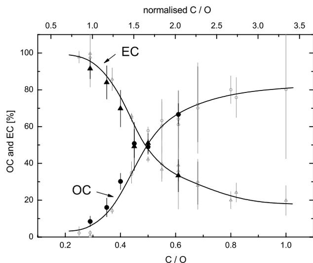
**Fig. 1.** Dependence of the particle composition (OC and EC content) on the C/O atomic ratio in the burner. Full symbols indicate measurements on samples from the NAUA chamber, open symbols indicate samples taken directly behind the CAST burner. The upper scale gives the C/O ratio normalised to the stoichiometric ratio of 0.3. The stoichiometric ratio separates fuel-lean (normalised C/O ratio < 1.0) and fuel-rich (normalised C/O ratio > 1) burner conditions.
