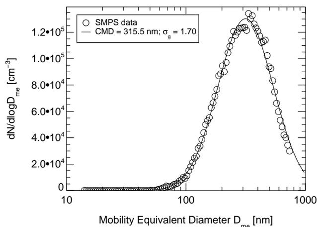
**Fig. 3.** Number size distribution of CAST aerosol produced at  $C/O=0.40$  and sampled from the chamber after the initial strong coagulation phase. The measured distribution is well reproduced by assuming lognormally distributed equivalent diameters.
