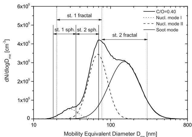
**Fig. 2.** Number size distribution measured by SMPS for an aerosol produced by the CAST at C/O=0.40. The vertical lines indicate the size ranges deposited on impactor stages 1 and 2 for the cases of compact spherical particles and fractal aggregates, respectively (see Sect. 4.1 and Sect. 4.2).
