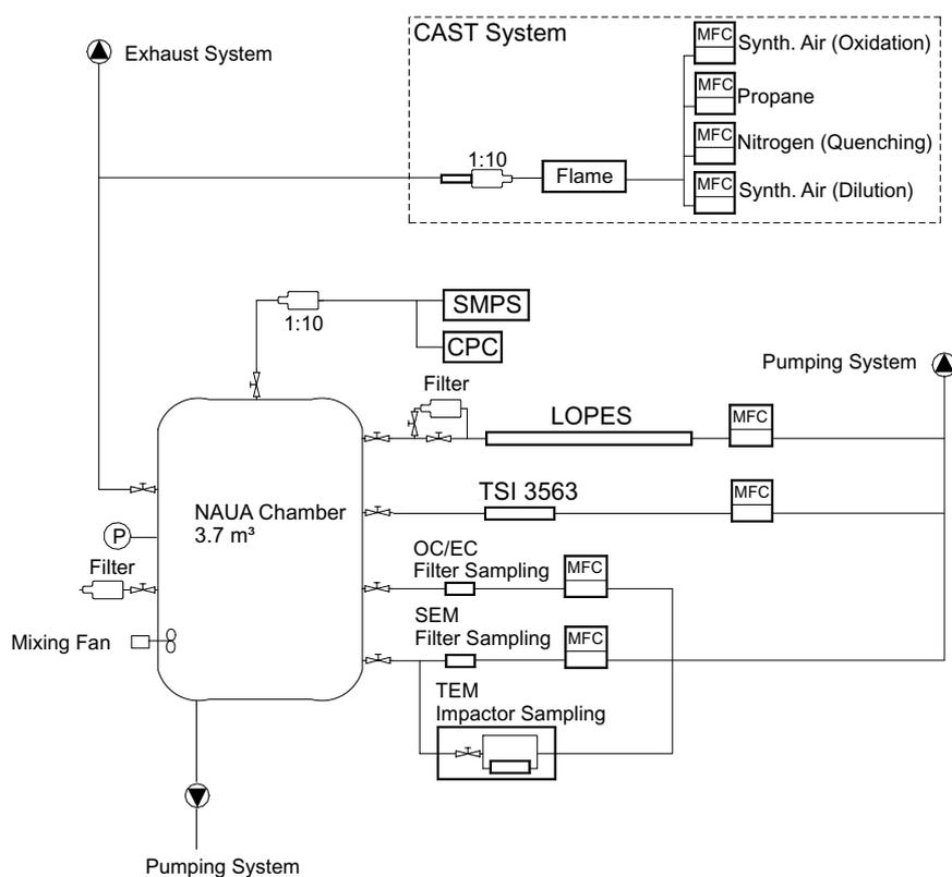
Fig. 5. Schematic representation of the aerosol chamber setup.
