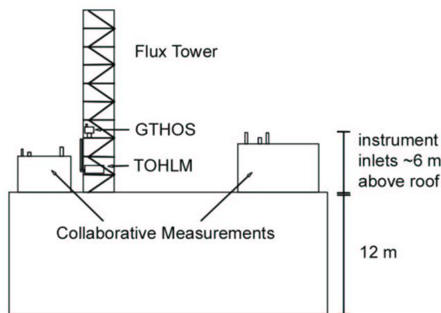
**Fig. 1.** Schematic of the instruments on the CENICA building roof. Both the Penn State instruments (GTHOS and TOHLM) were on the flux tower with their inlets within 1 m of one another. Collaborative measurements were also taken on the rooftop by other research groups.
