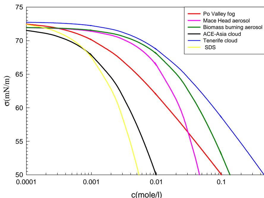
**Fig. 12.** Surface tension as a function of dissolved organic carbon concentration ( $c$ ) for fog, cloud and aerosol water extract samples from different environments. The curves were calculated with Eq. (14) (Syszkowski-Langmuir equation) and the data shown in Table 5 from data on real samples (cloud or fog droplets and aerosol water extracts).
