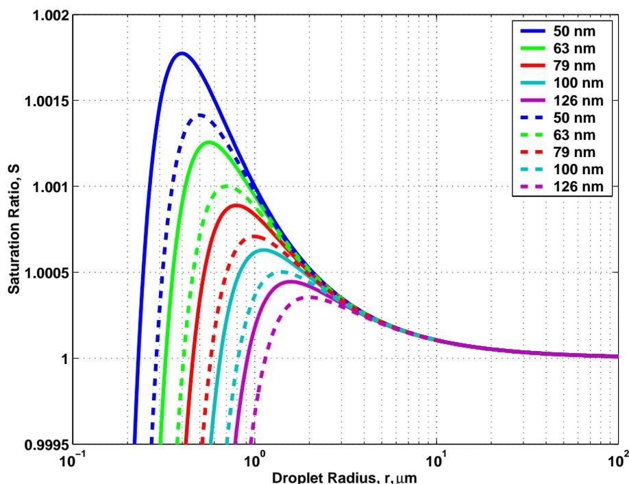
**Fig. 11.** Köhler curves calculated using Eq. (2) with surface tension reduction calculated using the  $\pi - A$  isotherm for stearic acid with 30% mass fraction solute stearic acid and 70%  $(\text{NH}_4)_2\text{SO}_4$ . Solid curves include surfactant, dashed are pure  $(\text{NH}_4)_2\text{SO}_4$ .
