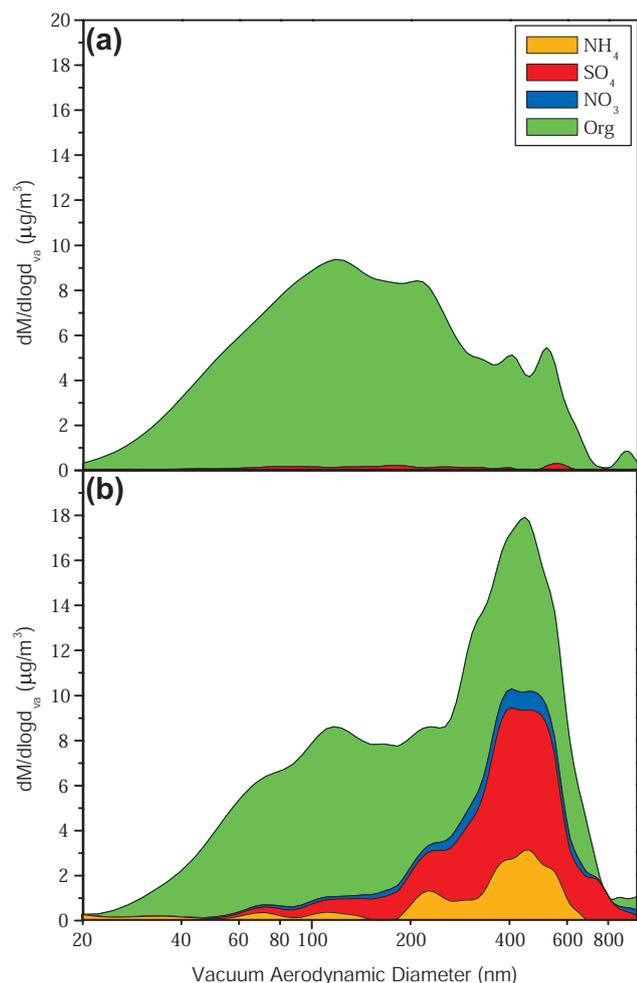
**Fig. 3.** AMS TOF spectra for two days showing mass concentrations vs. vacuum aerodynamic diameter. Green represents the organic fraction, red represents sulfate, blue represents nitrate, and orange represents ammonium. For example, the organic fraction in (b) at  $0.5 \mu\text{m}$  is approximately  $7 \mu\text{g}/\text{m}^3$ , not  $17 \mu\text{g}/\text{m}^3$ . (a) Hour 20:00–21:00 UTC, 5 September 2003. (b) Hour 16:00–17:00 UTC, 15 September 2003.
