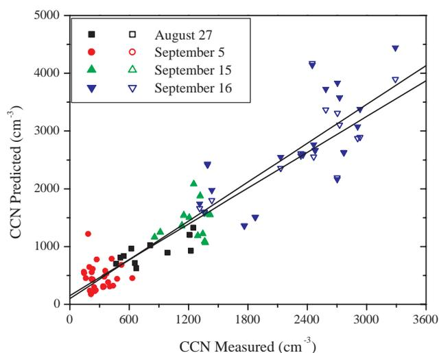
**Fig. 6.** Predicted CCN concentration vs. measured CCN concentrations for the four sample days. The filled symbols (■) are for predicted CCN concentrations based on the internally mixed assumption (see text). The open symbols (□) are for predicted CCN concentrations based on two particle modes on September 15 and 16 (see text). The black lines are linear least squares fits of the two data sets (slope=1.12±0.05; slope=1.03, ±0.05).
