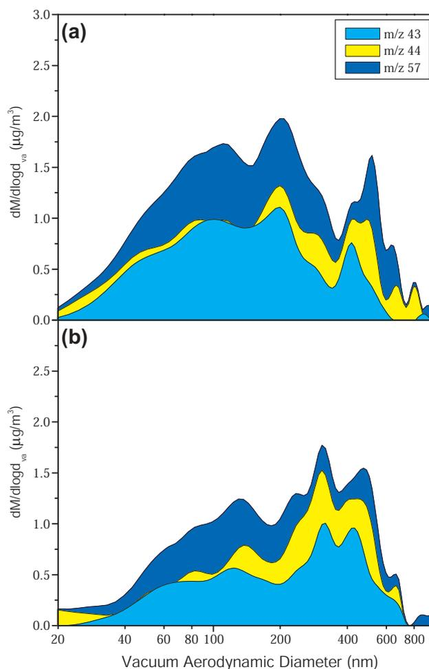
**Fig. 4.** AMS TOF spectra for two days showing key peaks in the organic mass fraction vs. vacuum aerodynamic diameter. The mass peak ( $m/z=44$  amu) is representative of aged organics, while the peak ( $m/z=57$  amu) is representative of primary emissions. The light blue represents  $m/z=43$ , the yellow represents  $m/z=44$ , and the dark blue represents  $m/z=57$ . (a) Hour 20:00–21:00 UTC, 5 September 2003. (b) Hour 16:00–17:00 UTC, 15 September 2003.
