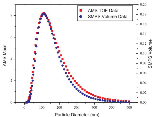
**Fig. 5.** Log-normal fits to the small mode, organic-rich fraction for 16:00–17:00 UTC, 15 September 2003. The red squares represent the fit to the AMS TOF data and the x-axis is  $D_{va}$ . The blue circles represent the fit to SMPS volume data and the x-axis is  $D_m$ .
