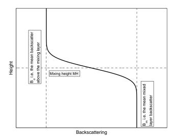
Fig. 1. An idealised backscattering profile.
