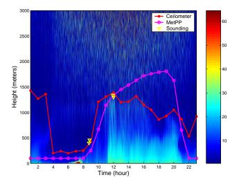
**Fig. 7.** A 24-h period of ceilometer echo intensity observations at Vantaa, 29 May 2002. The height of the MH determined by the ceilometer, the parcel method and the preprocessor (MetPP-FMI) are superimposed on the ceilometer raw echo data.
