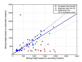
**Fig. 6.** Comparison between mixing heights determined by the ceilometer and radiosoundings (Holzworth method) in convective situations. Data points marked as hollow circles represent conditions with low backscattering signal.
