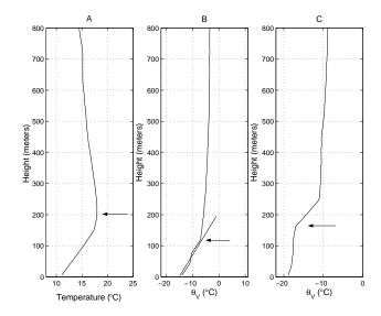
**Fig. 5.** Three ways for determining the reference mixing height from temperature profiles: (a) the height of the surface inversion (5 September 2002 06:06 UTC), (b) virtual potential temperature non-linearity (1 February 2002 07:02 UTC) and (c) strong winds – sharp virtual temperature increase above MH (2 January 2002 06:16 UTC).
