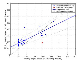
**Fig. 8.** Comparison between mixing heights determined by the ceilometer and radiosoundings (*Ri*-method) in stable situations (blue stars). The hollow circle corresponds to a case with low backscattering signal near the surface.
