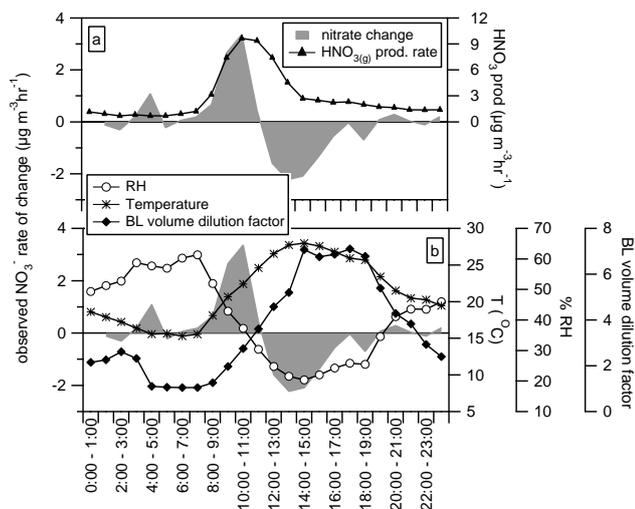
**Fig. 11.** Panel a: Diurnal production rate of  $\text{HNO}_3(\text{g})$  from Reaction (5) and observed rate of change of the mass concentration of nitrate. Panel b: diurnal cycles of RH, temperature and volume dilution factor of the BL.
