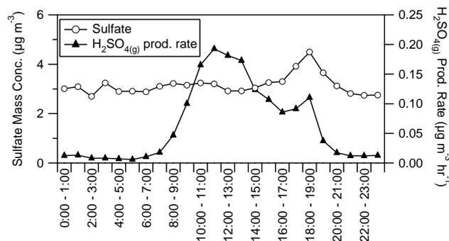
**Fig. 12.** Diurnal production rate of  $\text{H}_2\text{SO}_4(\text{g})$  from Reaction (6) and diurnal cycle of sulfate mass concentration. Averages were made over all time periods where sulfate,  $\text{SO}_2$  and OH data was available.
