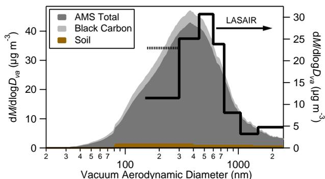
**Fig. 3.** Comparison of the (AMS + estimated BC + soil) and LASAIR size distributions. The BC, AMS and soil size distributions are stacked. The dashed line represents the mass concentration of the smallest LASAIR size channel multiplied by two in order to account for the 50% collection efficiency in this channel.
