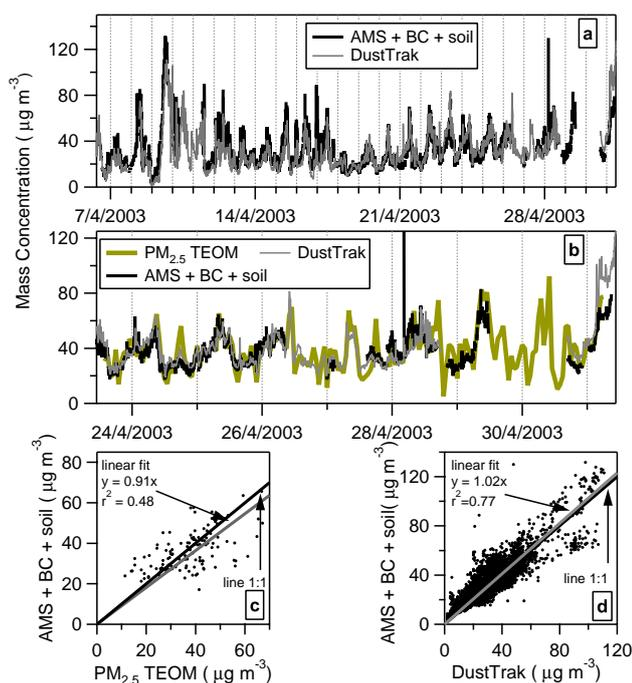
**Fig. 2.** Panels **a** and **b**: comparison of the time series of the AMS + BC + soil with DustTrak and TEOM PM<sub>2.5</sub> mass concentrations. Panels **c** and **d**: scatter plots and linear fits for the above comparisons. TEOM PM<sub>2.5</sub> data in panels **b** and **c**, has a resolution of 1 h; AMS + BC + soil data in panel **c** was averaged in 1 h periods. Grey lines are linear fits to the data. Lines 1:1 are shown in black as reference.
