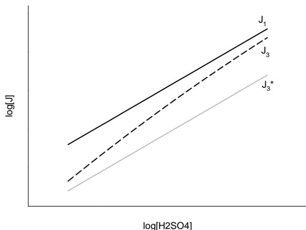
**Fig. 1.** Schematic dependence of apparent nucleation rate on sulphuric acid concentration.  $J_1$  is the particle formation rate at 1 nm,  $J_3$  the apparent particle formation rate at 3 nm and  $J_3^*$  the apparent particle formation rate at 3 nm if sulphuric acid does not participate in growth.
