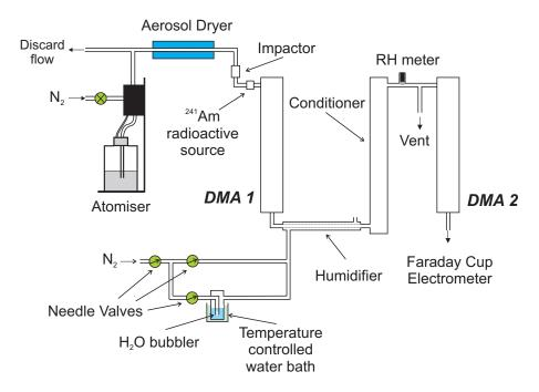
Fig. 2. Schematic of the experimental set-up for the TDMA experiments.
