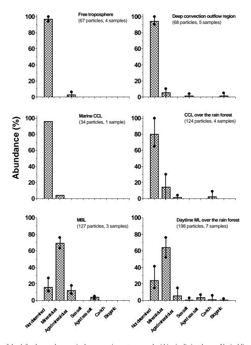
**Fig. 3.** Abundance of the defined aerosol groups in the super-micrometer aerosol within six distinct layers. Vertical lines indicate range of the abundances based on individual samples. In case the lowest observed abundance was zero, the lower limit dot is not displayed.
