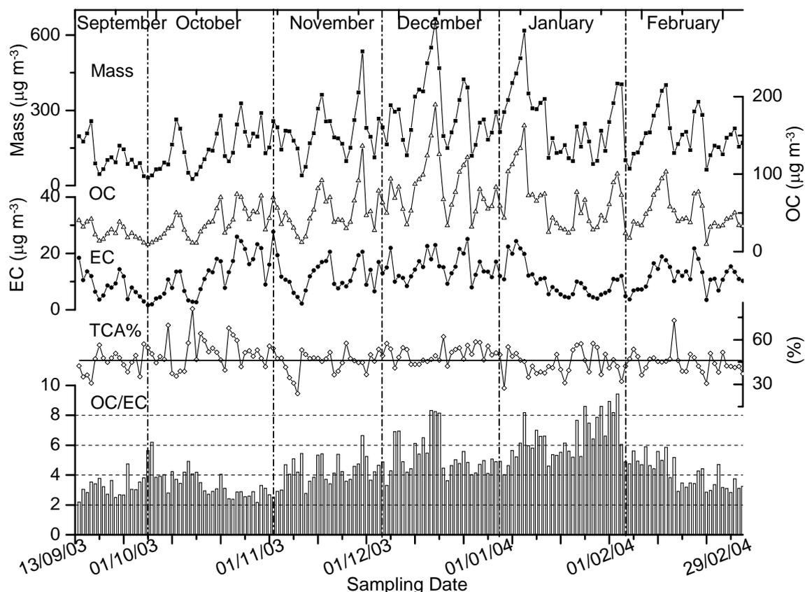
**Fig. 2.** Time series of  $PM_{2.5}$  mass, organic carbon (OC), elemental carbon (EC), fraction of  $PM_{2.5}$  composed of  $OC \times 1.6 + EC$  (TCA%), and OC/EC ratios at Xi'an from 13 September 2003 to 29 February 2004. OC is multiplied by 1.6 for the TCA% calculation to account for unmeasured hydrogen and oxygen in organic material (Turpin and Lim, 2001).
