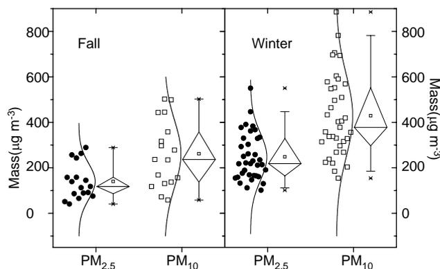
**Fig. 4.** Distribution of  $PM_{2.5}$  and  $PM_{10}$  mass concentrations during fall and winter. The valid paired samples were 17 in fall and 36 in winter. The box plots indicate the mean 24-h concentration and the min, 1st, 25th, 50th, 75th, 99th and max percentiles. A normal curve is fitted to the measurements.
