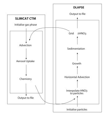
Fig. 1. Flow diagram illustrating the coupled DLAPSE/SLIMCAT model.
