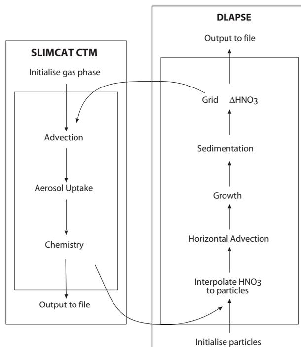
**Fig. 1.** Flow diagram illustrating the coupled DLAPSE/SLIMCAT model.
