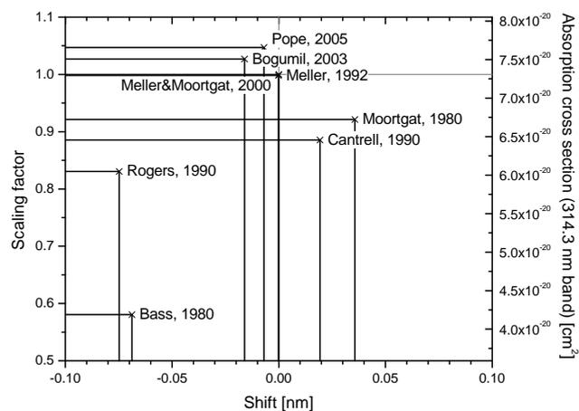
**Fig. 6.** Overview on the differences in magnitude and wavelength calibration of the available highly-resolved absorption cross-sections of formaldehyde with respect to the spectrum by Meller and Moortgat (2000).
