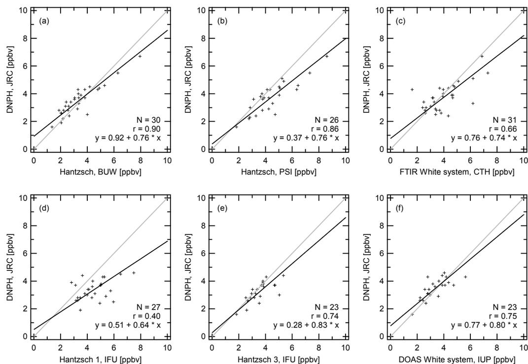
**Fig. 4.** Regressions of the DNPJ cartridge results from the intercomparison week plotted versus those from continuous techniques for concordant two hour time spans. The solid black line drawn through the data is the orthogonal least squares fit to the data (York, 1966). The grey line represents the one to one correspondence.
