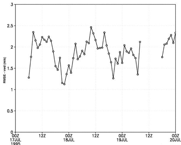
**Fig. 4.** Time series of the root-mean-square wind-vector-difference error (RMSE-vwd) for the near-surface wind field (10 m a.g.l.) as spatial average on all stations for simulation S<sub>1</sub> in grid G<sub>4</sub>. The corresponding temporal average value over the three-day period is 1.9 m/s.
