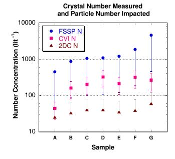
**Fig. 1.** Equivalent number concentration of particles collected on CVI electron microscope grids compared to number measured by the FSSP-100 and 2D-C probes for seven different samples. Error bars represent measurement uncertainty as described in the text. Due to the lengthy time required to perform the count, only seven of the total microscope samples were analyzed.
