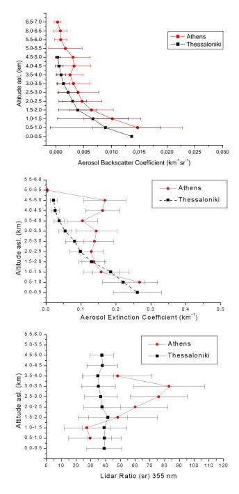
**Fig. 7.** The mean aerosol backscatter (**a**), extinction (**b**) and lidar ratio (**c**) profiles at 355 nm, obtained over Athens and Thessaloniki, Greece during the period 2000–2002. The standard deviation is also shown.
