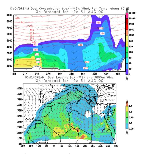
**Fig. 6.** Dust concentration  $(g/m^3)$  (upper part) and dust loading  $(g/m^2)$  (lower part) forecasted by the DREAM model for 31 August 2000 at 12:00 UT.
