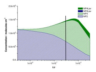
**Fig. 4.** The ratio of nitrophenols produced at 278 K as a function of  $L_c$  with the liquid phase reaction of NO<sub>3</sub> with phenol yielding (a) 90% 2-nitrophenol and 10% 4-nitrophenol and (b) 90% 4-nitrophenol and 10% 2-nitrophenol.
