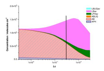
**Fig. 3.** The relative importance of the different nitration pathways at 278 K as a function of  $L_c$ .
