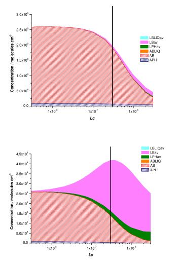
**Fig. 7.** The relative importance of the different nitration pathways at 298 K with the phenol + NO<sub>3</sub> liquid phase reaction rate coefficient set at (a)  $1.8 \times 10^8 \, \text{L mol}^{-1} \, \text{s}^{-1}$  and (b)  $1.8 \times 10^{10} \, \text{L mol}^{-1} \, \text{s}^{-1}$  (compare with Fig. 5 for rate coefficient of  $1.8 \times 10^9 \, \text{L mol}^{-1} \, \text{s}^{-1}$ ).
