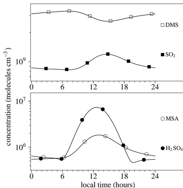
**Fig. 3.** Diurnal cycles of the concentrations ( $\text{molecules cm}^{-3}$ ) of DMS,  $\text{SO}_2$ , MSA, and  $\text{H}_2\text{SO}_4$  at the mean values of the parameters.
