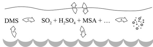
**Fig. 1.** Major processes affecting gas-phase DMS-related species in the clear-sky RMBL:  $e$ =emissions of DMS from the ocean,  $c$ =chemical oxidation,  $d$ =dry deposition,  $a$ =loss to background aerosols, and  $m$ =mixing in to and out of the RMBL.
