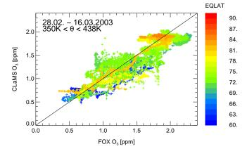
**Fig. 13.** Comparison of ozone mixing ratios simulated by CLaMS and observed by FOX on Geophysica between 28 February and 16 March 2003, The color of the symbols denotes the equivalent latitude of the observation location.
