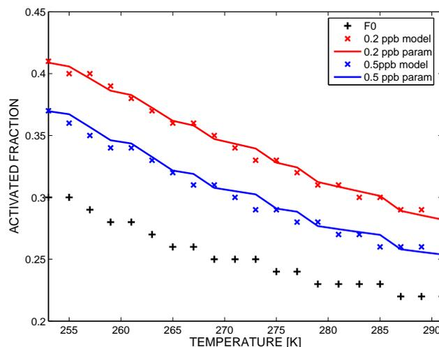
**Fig. 2.** Activated fraction as a function of temperature for three different HNO<sub>3</sub> concentrations as modeled by parcel model and corresponding predictions by new parameterization.
