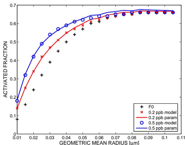
**Fig. 3.** Activated fraction as a function of geometric mean radius as modeled by parcel model and corresponding predictions by new parameterization when  $V=0.5$  m/s,  $N=1000$  cm<sup>-3</sup> and  $\sigma=1.8$ .
