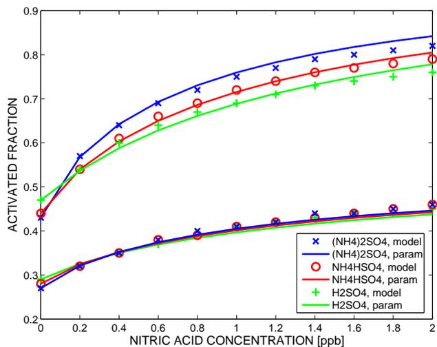
**Fig. 5.** Activated fraction as a function of aerosol particle number, nitric acid concentration and aerosol particle chemical composition. In the upper set of lines total  $N=400 \text{ cm}^{-3}$  and in the lower set  $N=2000 \text{ cm}^{-3}$ .
