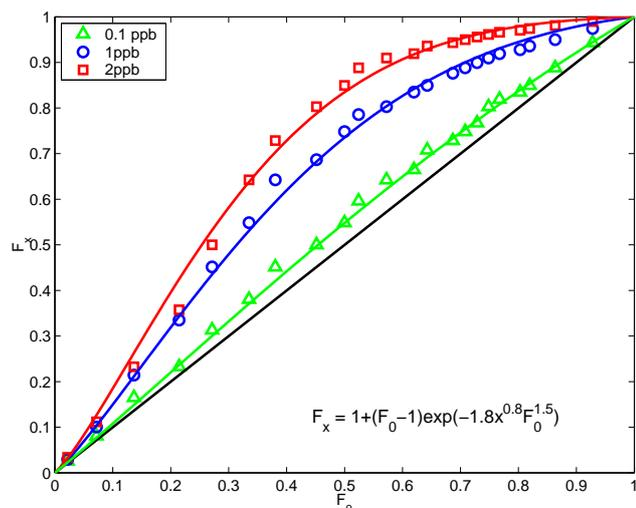
**Fig. 1.**  $F_x$  as a function of  $F_0$  for three different HNO<sub>3</sub> concentrations and lines are calculated with fitted Eq. (2).
