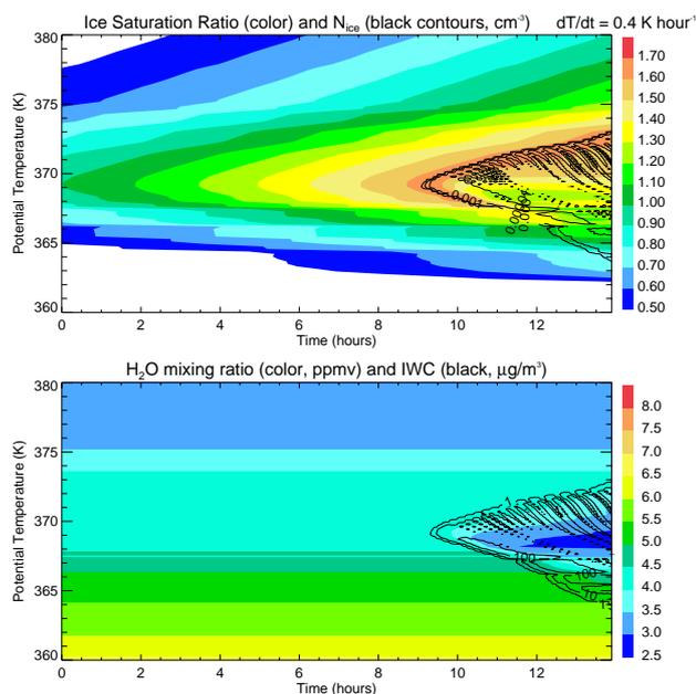
**Fig. 2.** Color shading shows saturation ratio (top panel) and water vapor mixing ratio (bottom panel) versus time and height for an idealized simulation with a column of air cooling over several hours leading up to the WB-57 sampling time. Location of the ice cloud is indicated by black ice number density contours. The cloud formation limits the ice saturation ratio to  $\leq 1.65$  and dehydrates the region near the tropopause.
