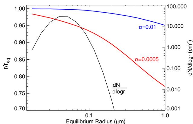
**Fig. 5.** The ratio of aerosol radius divided by the equilibrium radius is plotted versus equilibrium radius for different accommodation coefficients (red and blue curves). The aerosol size distribution used in the simulations is shown for reference. If  $\alpha_c$  is significantly decreased by surface impurities, the aerosols can be much more concentrated and less likely to freeze than they would be in equilibrium with the vapor.
