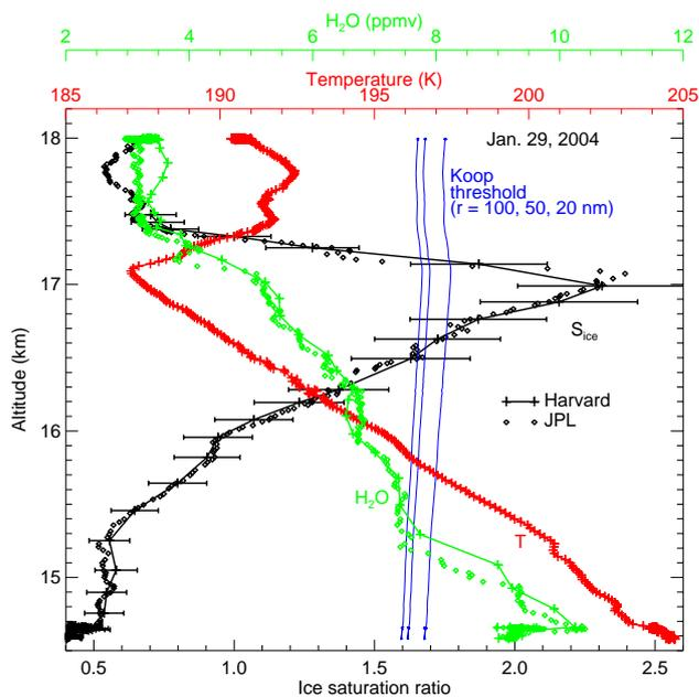
**Fig. 1.** In situ measurements from a WB-57 descent across the cold tropopause south of Costa Rica are shown. Ice supersaturations at the tropopause are far larger than the threshold for ice nucleation due to freezing of aqueous aerosols (in equilibrium with the ambient water vapor) indicated by a measurement-based parameterization (Koop et al., 2000) (blue curves). See text for discussion.
