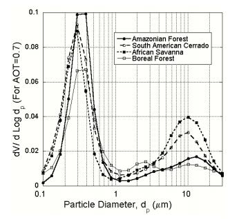
**Fig. 2.** Retrieved AERONET particle size distributions for a 440 nm Aerosol Optical Depth (AOT) of 0.7.
