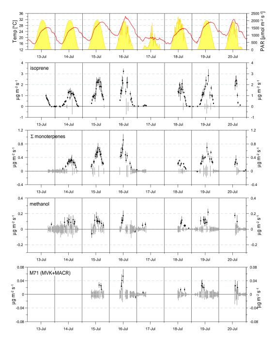
Fig. 8a. Fluxes of BVOCs at the west tower. Black error bars are the precisions of individual flux measurements, grey error bars denote the confidence interval in the cases where no fluxes could be determined.
