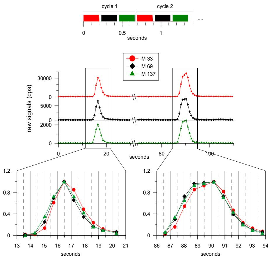
**Fig. 3.** Measurements of two concentration pulses as generated by aspirating a standard gas through the 60 m long inlet lines. Top: visualisation of the sequential measurement of the three masses within one measurement cycle, middle: raw signals of the PTR-MS, and bottom: peaks normalised to maximum concentration.
