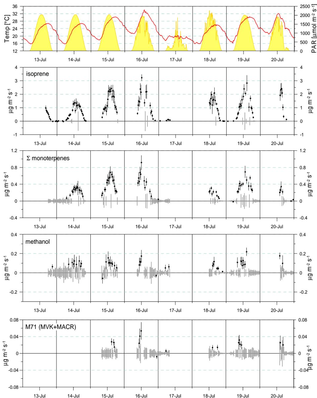
**Fig. 8a.** Fluxes of BVOCs at the west tower. Black error bars are the precisions of individual flux measurements, grey error bars denote the confidence interval in the cases where no fluxes could be determined.
