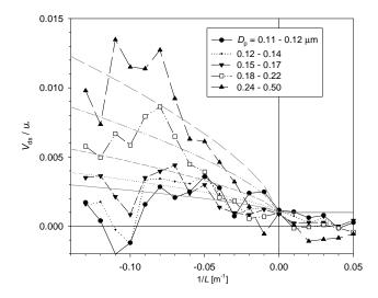
**Fig. 3.** Normalized values of the measured deposition velocity  $(V_{ds}/u_*)$  as a function of the stability parameter  $(L^{-1})$  for five ranges of particle diameter  $(D_p)$ . Theoretically predicted curves according to Eq. (12) are also shown (grey lines).
