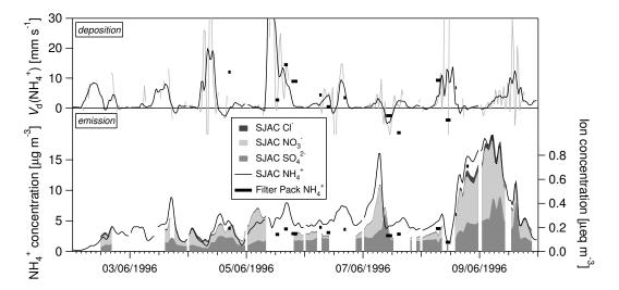
**Fig. 4.** Example time series of  $NH_4^+$  concentrations and deposition velocities ( $V_d$ ) derived by gradient method from the SJAC and filter-pack data. For the SJAC both 30-min measurement data (thin grey) and a 3-h running mean (bold black) are shown. Also shown are the equivalent concentrations of the main anions associated with  $NH_4^+$  ( $SO_4^{2-}$ ,  $NO_3^-$  and  $Cl^-$ ).
