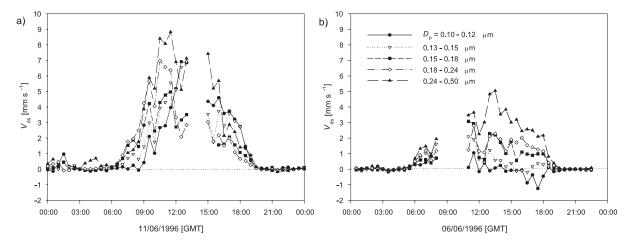
**Fig. 2.** Example daily courses of the deposition velocity of five size classes of particles as measured by eddy-covariance with the ASASP-x. In case (a) particles of all sizes are continuously deposited, at a rate that increases with particle size, whereas (b) on 6 June apparent emission of small particles was observed in the afternoon.
