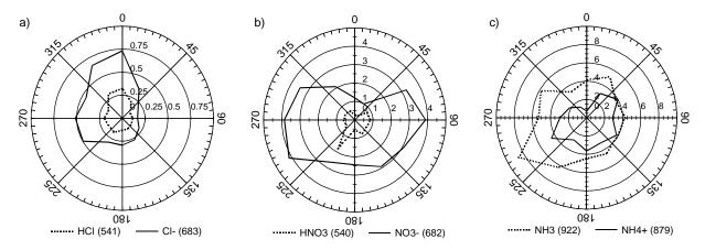
**Fig. 1.** Wind-sector dependencies of median concentration ( $\mu$ g m<sup>-3</sup> as Cl and N) of (**a**) HCl and Cl<sup>-</sup> aerosol, (**b**) HNO<sub>3</sub> and NO<sub>3</sub><sup>-</sup> aerosol, as well as (**c**) NH<sub>3</sub> and NH<sub>4</sub><sup>+</sup> measured at Elspeet, with the number of observation provided in parentheses.
