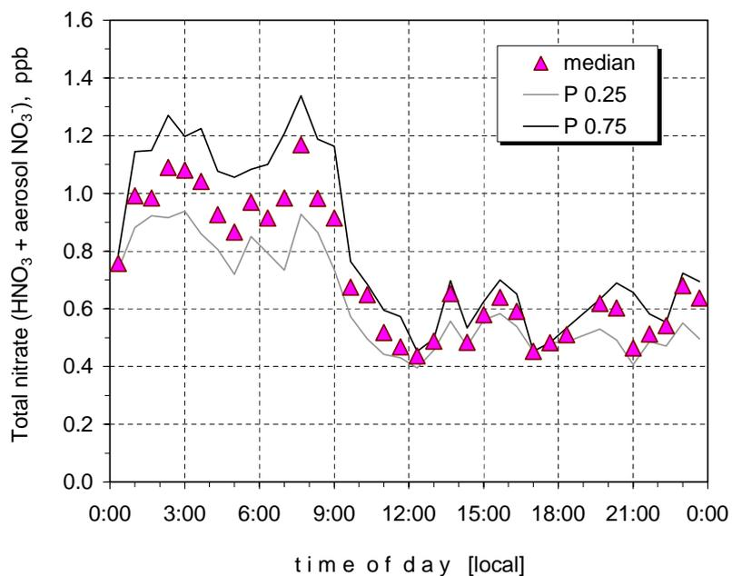
**Fig. 11b.** Median diel variation of total nitrate (aerosol NO<sub>3</sub><sup>-</sup> + HNO<sub>3</sub>) covering a period during the biomass burning season (17–20 Sep.) at FNS during SMOCC 2002.
