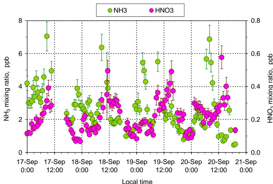
**Fig. 6.** Diel variations of  $\text{NH}_3$  and  $\text{HNO}_3$  from 17 to 20 September (biomass burning season) at FNS during SMOCC 2002. Error bars indicate measurement uncertainty for each data point.
