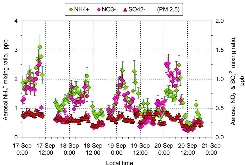
**Fig. 9a.** Diel variations of aerosol  $\text{NH}_4^+$ ,  $\text{NO}_3^-$  and  $\text{SO}_4^{2-}$  (fine fraction,  $D_p \leq 2.5 \mu\text{m}$ ) from 17 to 20 September (biomass burning season) at FNS during SMOCC 2002. Error bars indicate measurement uncertainty for each data point.
