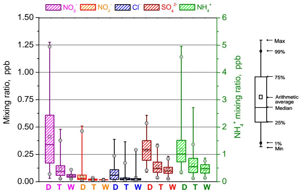
**Fig. 5.** Box-and-whisker plots showing seasonal mixing ratio variations of aerosol species during dry season (D), transition period (T) and wet season (W) at FNS during SMOCC 2002. Aerosol measurements of bulk and fine fraction ( $D_p < 2.5 \mu\text{m}$ ) were included.
