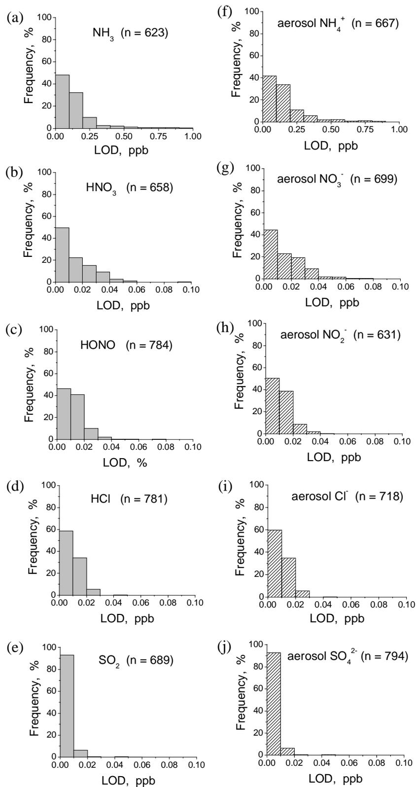
**Fig. 3.** (a–j). Limit of detection (LOD) frequency distributions (given as atmospheric mixing ratios) of gaseous (a–e) and aerosol (f–j) species measured at FNS during SMOCC 2002 (n=total number of values).
