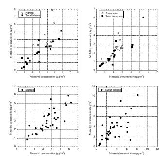
**Fig. 6.** Comparison of simulated and measured annual averaged concentrations of the inorganic aerosol components.
