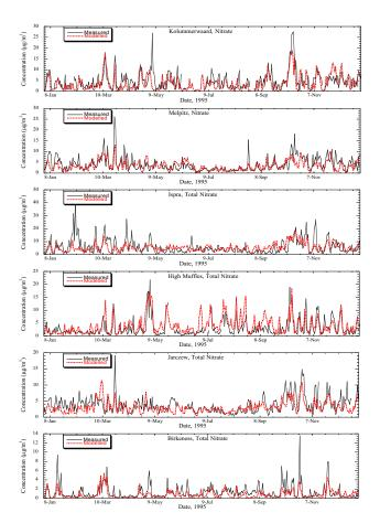
**Fig. 8.** Modelled and measured time series of nitrate and total nitrate over 1995.
