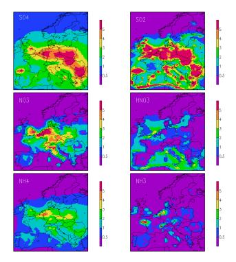
**Fig. 3.** Annual average concentrations ( $\mu$ g/m<sup>3</sup>) of inorganic aerosols and their precursor gases at measuring height.
