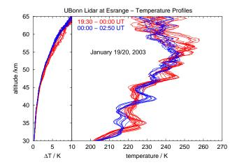
**Fig. 4.** Temperature profiles for 19/20 January 2003 measured by the ALOMAR RMR lidar (left plot) and the U. Bonn lidar (right plot). Shown are temperature profiles of 1 h integration time. The starting points of the integrations are shifted by 15 min. The left part of each plot presents the temperature errors for each individual profile.
