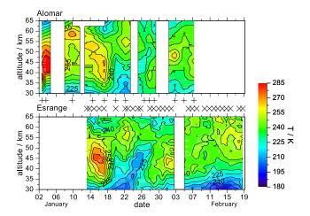
**Fig. 1.** Evolution of the nightly mean temperatures as observed by the ALOMAR RMR lidar in Norway (upper row) and the U. Bonn lidar at the Esrange in Sweden (lower row) for January and February 2003. The abscissa shows the date of January/February 2003, the ordinate the altitude in kilometers, and the color code the temperature in Kelvin. Measurement times are marked by "+"-signs for ALOMAR data and "×"-signs for Esrange data
