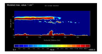
**Fig. 5c.** Modeled Nucleation Mode particle concentration (cm<sup>-3</sup>) after 3 h simulation. The modeled value at 10.4 km is indicated in the figure.
