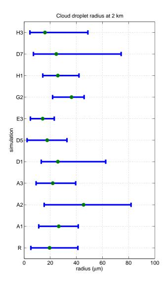
**Fig. 11a.** Average (both horizontally and over 3 h of simulation) effective cloud droplet radius at cloud base (2.0 km). Also shown in the figure are the maximum and minimum horizontally averaged effective cloud droplet radius simulated over the 3-h period.
