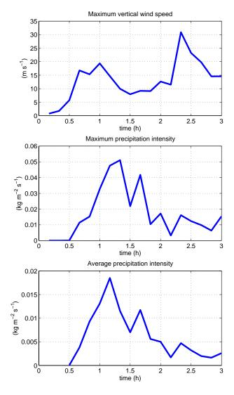
**Fig. 4.** Time development of simulated maximum vertical wind velocity, maximum precipitation and model domain average precipitation.
