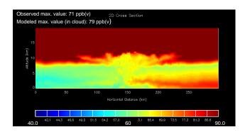
**Fig. 5i.** Modeled O<sub>3</sub> concentration (ppb) after 3 h simulation. Modeled and observed values at 10.4 km are indicated in the figure.
