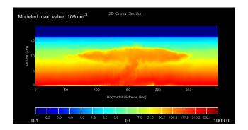
**Fig. 5g.** Modeled BC Mode particle concentration (cm<sup>-3</sup>) after 3 h simulation. The modeled value at 10.4 km is indicated in the figure.
