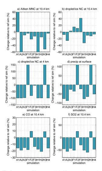
**Fig. 6.** Percentage difference at t=3 h in (a) average Aitken mode particle number concentration at 10.4 km, (b) ice/droplet particle number concentration at 10.4 km, (c) ice/droplet particle number concentration at 4 km, (d) average surface precipitation, (e) average CO concentration at 10.4 km and (f) average SO<sub>2</sub> concentration between reference simulation and sensitivity simulation series A, F and H.
