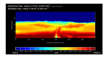
**Fig. 5d.** Modeled Aitken Mode particle concentration (in  $100 \,\mathrm{cm}^{-3}$ ) after 3 h simulation. Modeled and observed values at  $10.4 \,\mathrm{km}$  are indicated in the figure.
