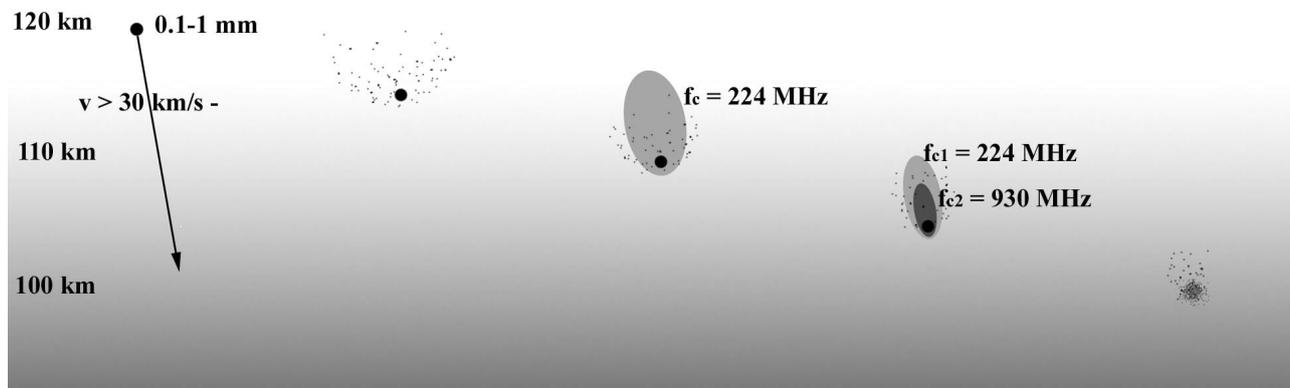
**Fig. 3.** The meteor head echo appears first at the VHF as the target reaches the critical density and a few kilometres lower down at the UHF as the target plasma is compressed further to the corresponding critical density.
