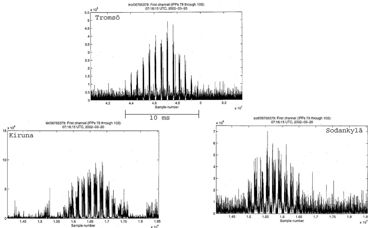
**Fig. 5.** Tristatic meteor observation with the EISCAT UHF radar. The vertical axes show in arbitrary units the returned power in the scattering process from the meteor head. The meteor is seen from three different directions (Kiruna, Tromsø and Sodankylä) when it passes the radar beam.
