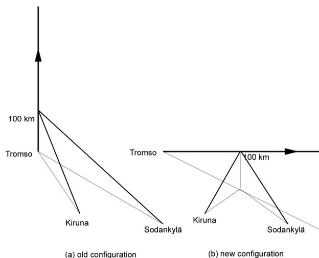
**Fig. 4.** The EISCAT tristatic measurement geometry. During the first experiments the Tromsø beam was vertical and the remotes were pointing to it at about 105 km altitude (a). (b) shows the optimised geometry to get highest possible tristatic rates.
