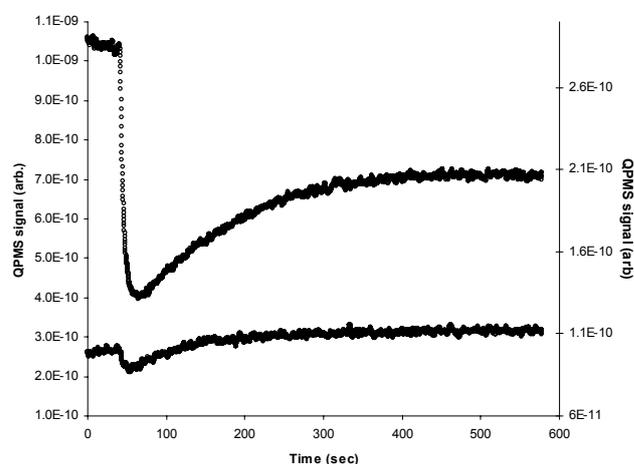
**Fig. 5.** An example of a typical Knudsen experiment performed with a steady state flow. Steady state concentrations of SO<sub>2</sub> and NO<sub>2</sub> were 5.0×10<sup>12</sup> and 1.0×10<sup>13</sup> molecules cm<sup>-3</sup>, respectively. The top line represents the signal for SO<sub>2</sub> (m/z=64) and belong to the left y-axis. The lower line represents the signal for NO<sub>2</sub> (m/z=46) and belong to the right y-axis.
