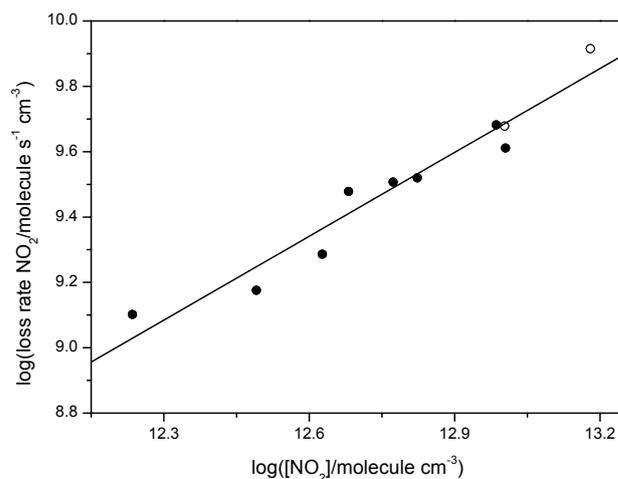
**Fig. 7.** Bilogarithmic plot of the loss rate of  $\text{NO}_2$  as a function of  $[\text{NO}_2]$ . Filled circles are from experiments with both  $\text{SO}_2$  and  $\text{NO}_2$  present, open circles are from experiments with only  $\text{NO}_2$ . The reaction order was determined to be  $n=0.85\pm 0.28$  ( $2\sigma$ ),  $r^2=0.90$ , from linear regression of the experiments with  $\text{SO}_2$  and  $\text{NO}_2$  present (filled circles).
