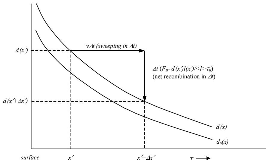
**Fig. 3.** Mechanism by which creation-recombination and the sweeping flux due to growth increases the D concentration  $d(x)$  near the surface. In time  $\Delta t$  growth adds a layer of thickness  $v\Delta t$ , thus effectively sweeping charge  $d(x')$  at point  $x'$  a distance  $\Delta x' = v\Delta t$  from the surface. In this time, net recombination removes an amount  $\Delta t(F_B - d(x')l(x')/\langle l \rangle \tau_B)$ .
